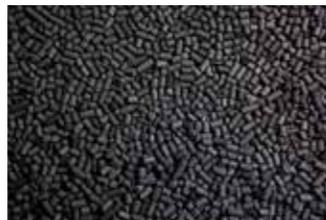
**IMPREGNATED ACTIVATED CARBONS:** In order to economically remove certain gas impurities which are difficult to adsorb, such as hydrogen sulphide, mercury or ammonia, the activated carbons can be markedly improved by suitable impregnation. The impurities are no longer removed by adsorption but by chemisorption. Typical impregnating chemicals are sulphur (mercury), potassium iodide
